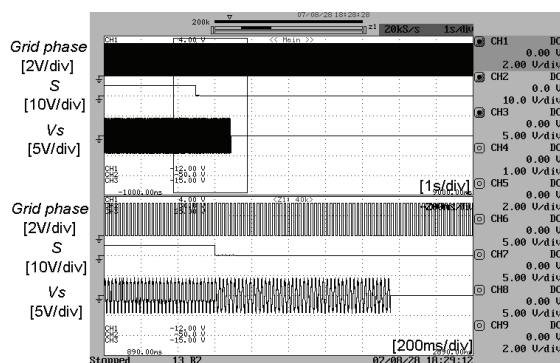
Figure 7: Observed waveforms at the experiment of the grid phase changes from 50[Hz] to 48[Hz] steeply
