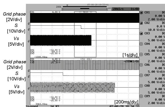
Figure 6: Observed waveforms at the experiment of the grid phase changes from 50[Hz] to 52[Hz] steeply
