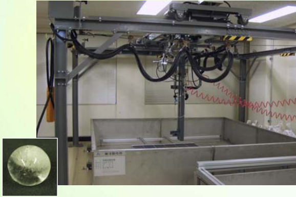
Hail Impact Test Equipment (23m/s, 25mm \phi Ice ball)
