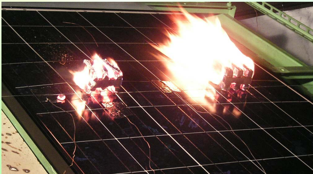
Fire Brand Test according to fire class B
