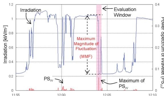
Fig. 1 Calculation image of MMF.
