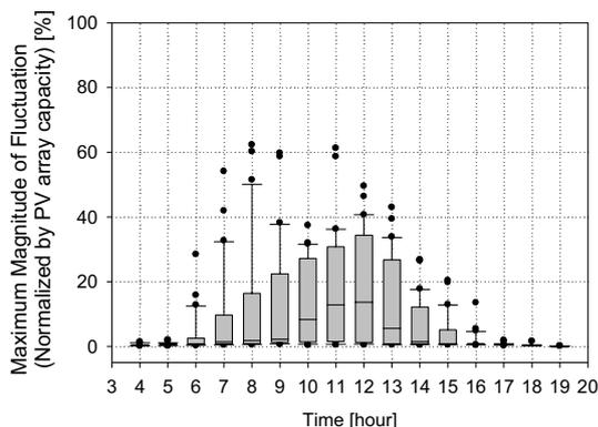
Fig. 2 MMF of System I (single array oriented east) of from two to four seconds fluctuation time.
