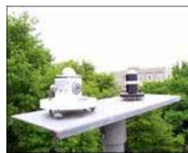
Fig. 6. Picture of experimental equipments for the development of the dual sensor pyranometer
