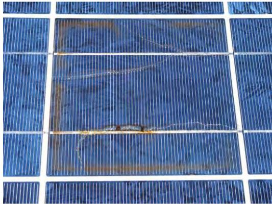
**Figure 6:** An Infrared thermal image and photo of the broken cell in the module
