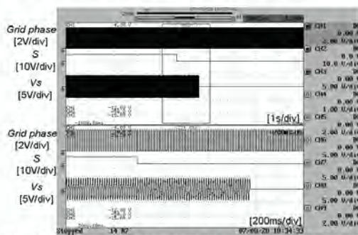
Figure 6: Observed waveforms at the experiment of the grid phase changes from 50[Hz] to 52[Hz] steeply
