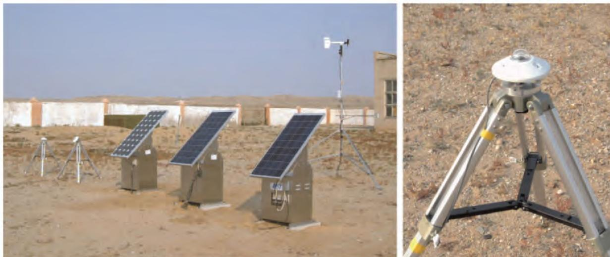
Figure 1. Overview of the experimental setup and horizontal pyranometer
