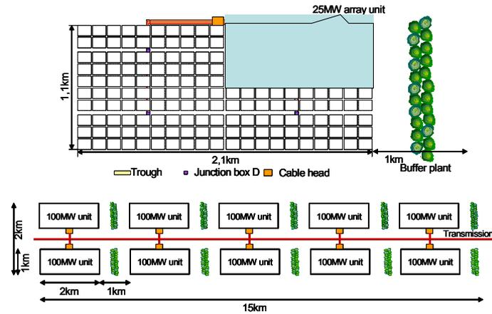
Fig. 2 Concept of 1GW PV array layout
