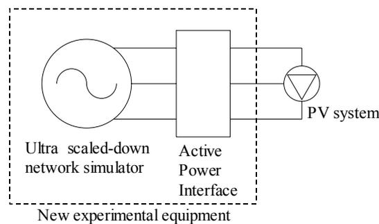
Fig. 1 Basic design of new type experimental equipment.
