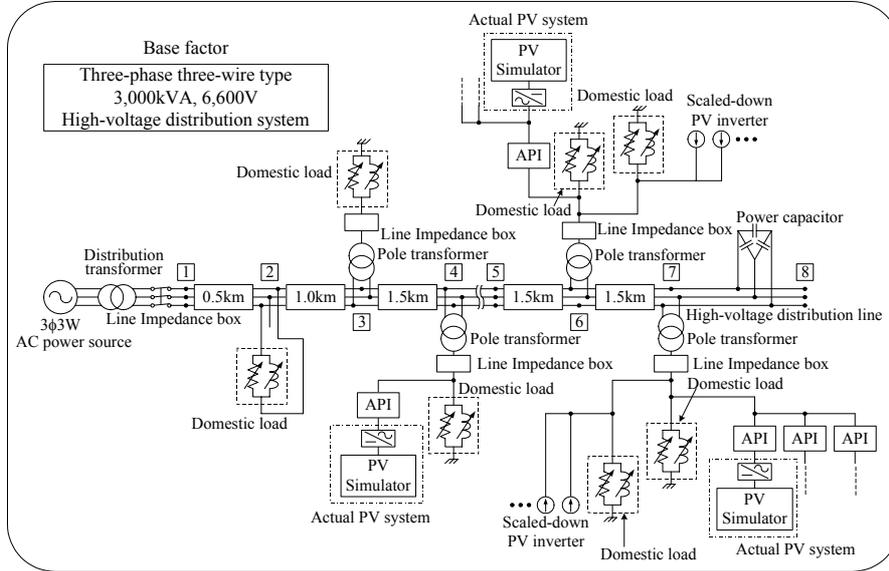
Fig. 2 Composition of the ultra scaled-down network simulator (residential area).
