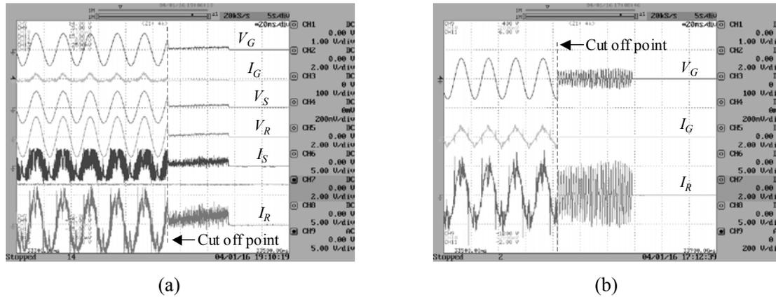
Fig. 6 Experimental results; (a) with API; (b) without API
