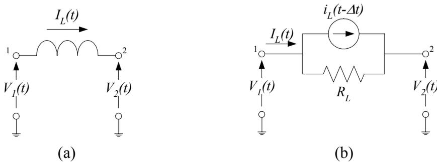
Fig. 4 (a) A inductance element; (b) an equivalent circuit of the inductance.
