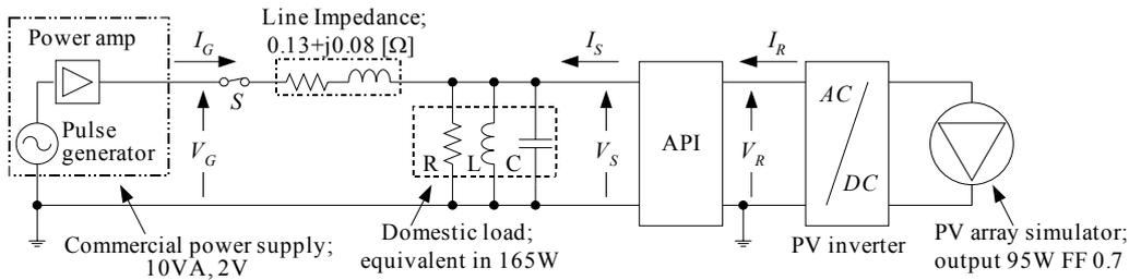
Fig. 5 An ultra scaled-down low voltage distribution system of single-phase two-wire type.
