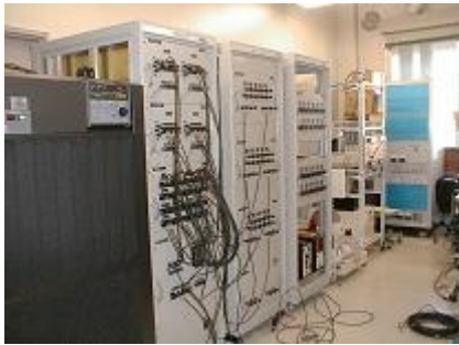
Figure 5: The reduced scale distribution system simulator.
