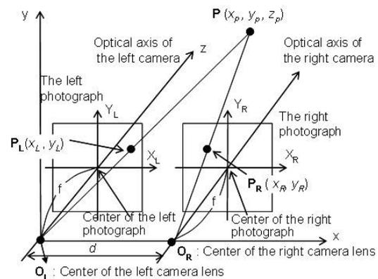
Fig.1 Calculation of the coordinates by triangulation
