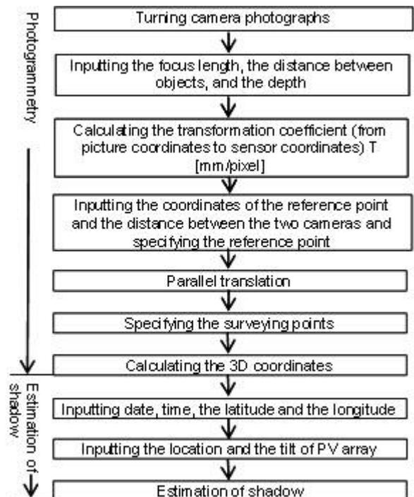
Fig.8 Flow of photogrammetry and estimation of shadow
