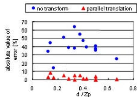
Fig.7 Estimation of errors of y coordinates by using the parallel camera images
