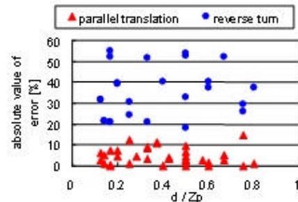
Fig.6 Estimation of errors of y coordinates by using the turning camera images
