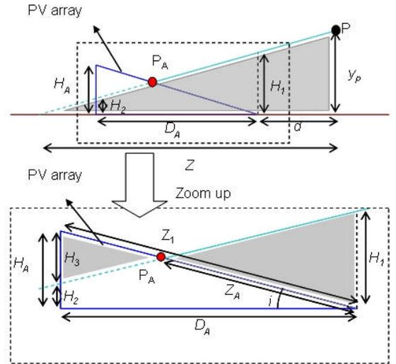
Fig.4 Side view of PV array in fig.3
