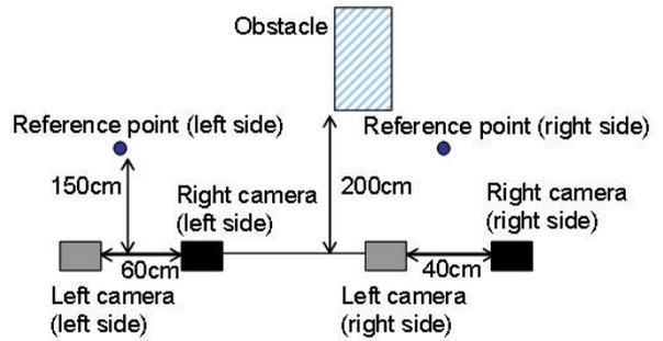
Fig.9 Schematic diagram of photogrammetry and the condition
