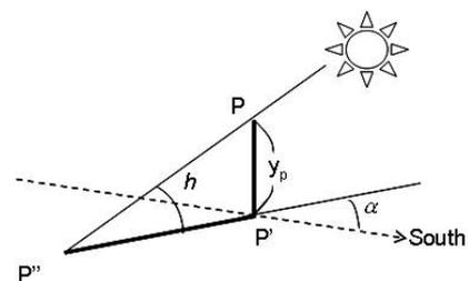
Fig. 2 Conceptual diagram of estimating shadows
