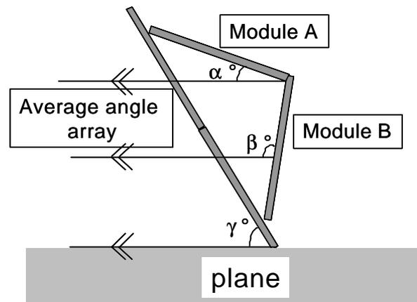
Fig. 11. Image of array configuration used in calculation
