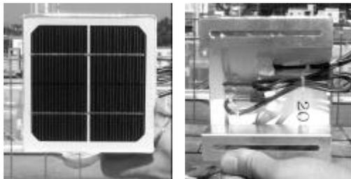
Fig. 3. Mini-module consisting of two-cells
