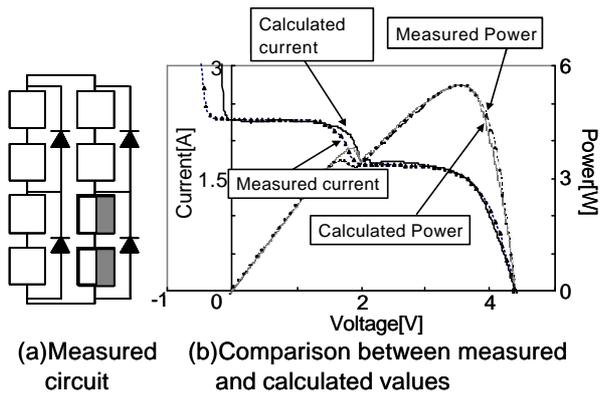
Fig. 10. Comparison between measured and simulated data
