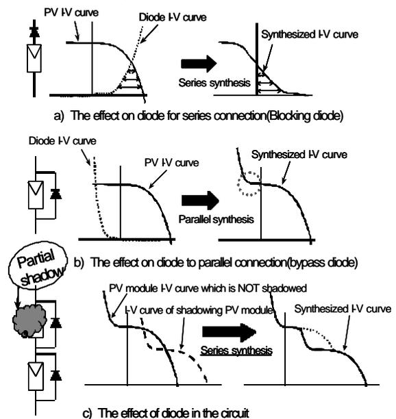
Fig. 5. The influence on diodes for 2cell module
