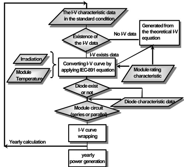
Fig. 1. The flowchart of the simulation model for simplified I-V curve interpolation method.
