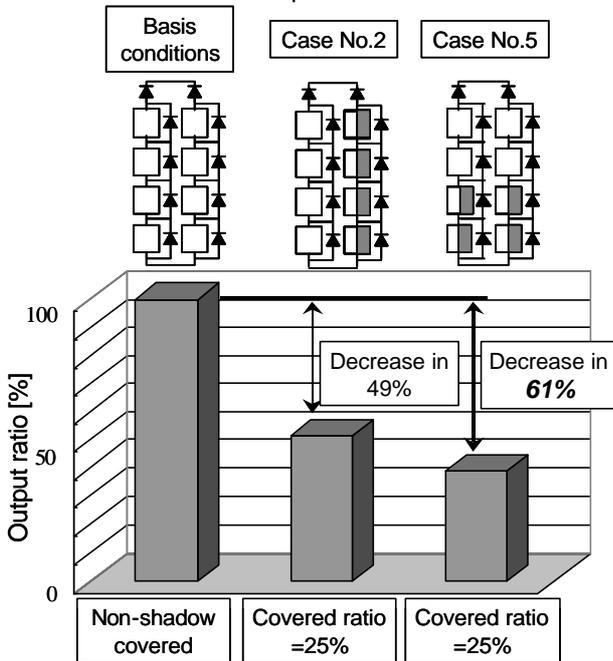
Fig. 7. Comparison of PV array power generation for experimental cases
