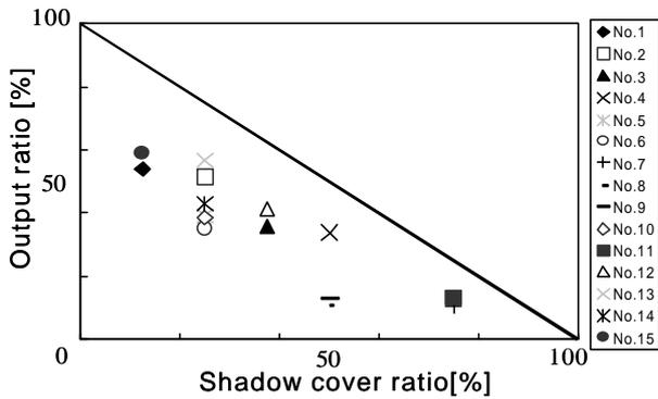
Fig. 6 Relationship between partial shadow patterns and PV power ratio
